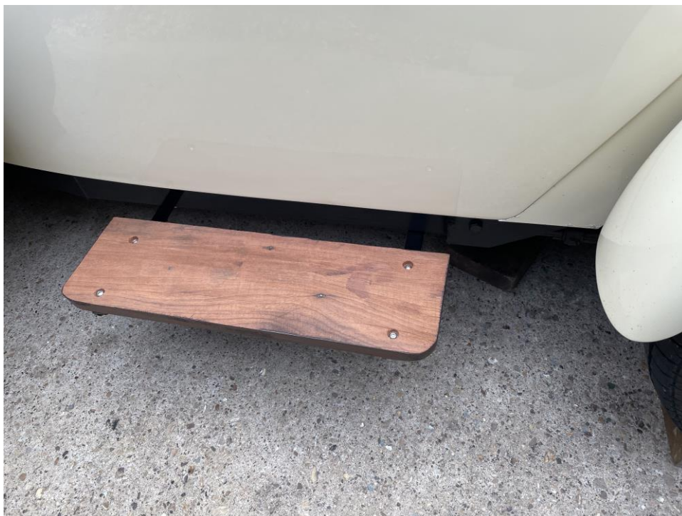
The passenger side trial fitted prior to removal for fitment of ribbed rubber covering.
